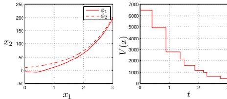
Fig. 4. Solutions of an unstable first order system on the cascade network topology from  $x_1(0,0) = (-5, 0)$   $x_2(0,0) = (10, 0)$  and  $\tau(0,0) = 0, 4$ . While the solutions themselves do not converge to anything, the Lyapunov function along the solutions decreases to zero, implying that solutions converge to each other asymptotically.
