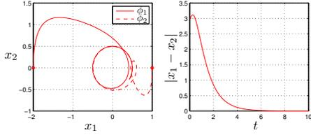
(a) The distance between the solutions using continuous control decreases to zero, implying that solutions synchronize asymptotically.
