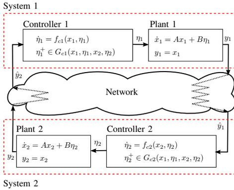
Fig. 2. Two continuous-time systems (plants) with dynamic controllers given by (4) for synchronization over a network with intermittent communication events. While  $G_{ci} : \mathbb{R}^n \rightrightarrows \mathbb{R}^p$  is a set-valued map updating the state of the controller when new information arrives. The resulting closed-loop system has the following dynamics:<sup>1</sup>
