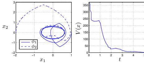
Fig. 3. Solutions to a coupled harmonic oscillator system on the feedback network topology from  $\hat{x}_1(0,0) = (1, 0, 0, 0.2)$   $\hat{x}_2(0,0) = (-2, 0, 0, -0.1)$ . (right) On the  $x_1, x_2$ -planar perspective the solutions converge to a circular orbit about the origin, (left) the Lyapunov function along the solutions decreases to zero, implying that solutions converge to each other asymptotically.
