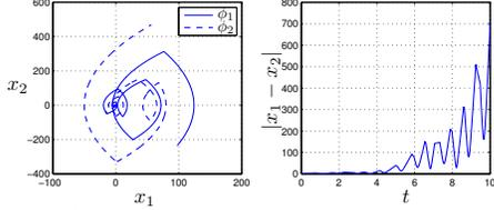
(b) With  $t_{k+1}^i - t_k^i \in [0.5, 1]$  for  $i \in \{1, 2\}$ ,  $k \in \mathbb{N} \setminus \{0\}$ , the intermittent communication prevents the controller from steering the distance between solutions to zero.
